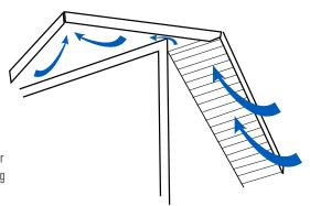
ICC guidelines recommends that the free area of ventilation (in square inches) needed is the number at which the two columns intersect. The sum of the free area of all ceilings equal the total free area required. The total square feet of an attic space divided by 300 = the total net free area required for appropriate ventilation.
